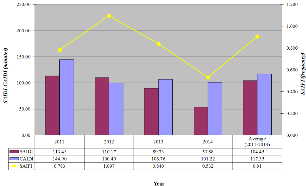
Figure 9.2 Lewistown system indices including major event days (MEDs) as defined in IEEE Standard 1366-2012.
