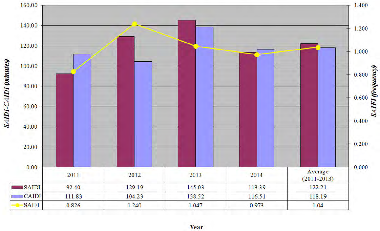
Figure 5.2 Butte system indices including major event days (MEDs) as defined in IEEE Standard 1366-2012.
