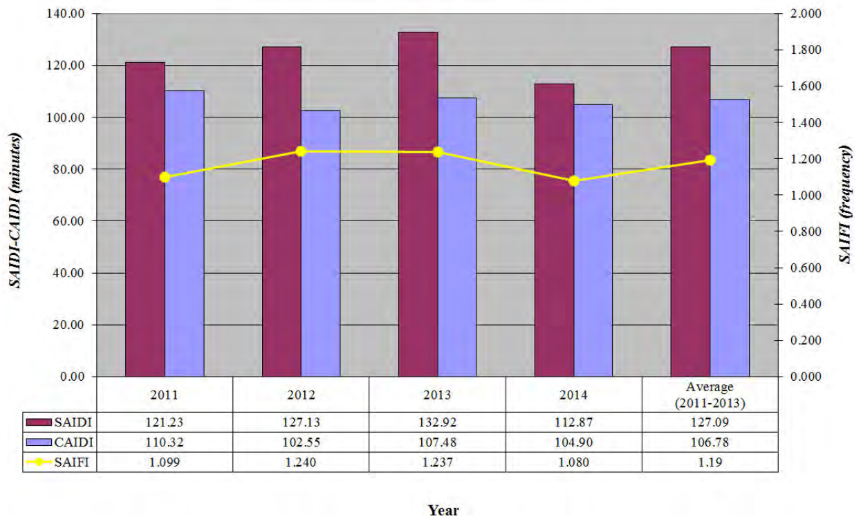
Figure 2.1 Montana system indices excluding major event days (MEDs) as defined in IEEE Standard 1366-2012.
