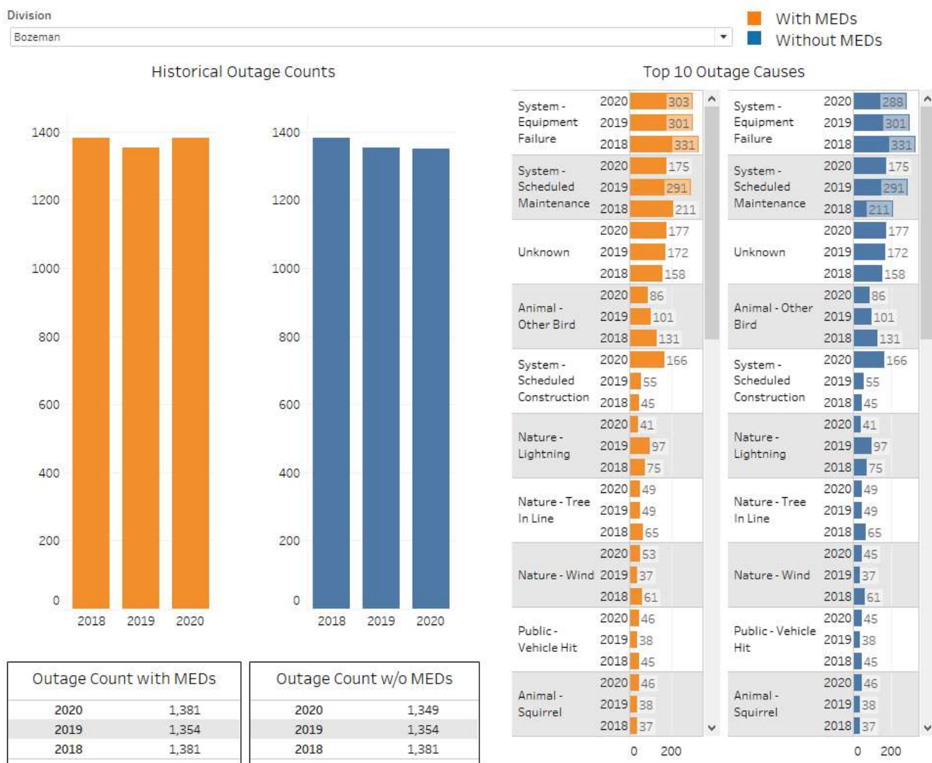
Figure 4.2 Bozeman system outages by top ten causes with and without major event days (MEDs) as defined in IEEE Standard 1366-2012.
