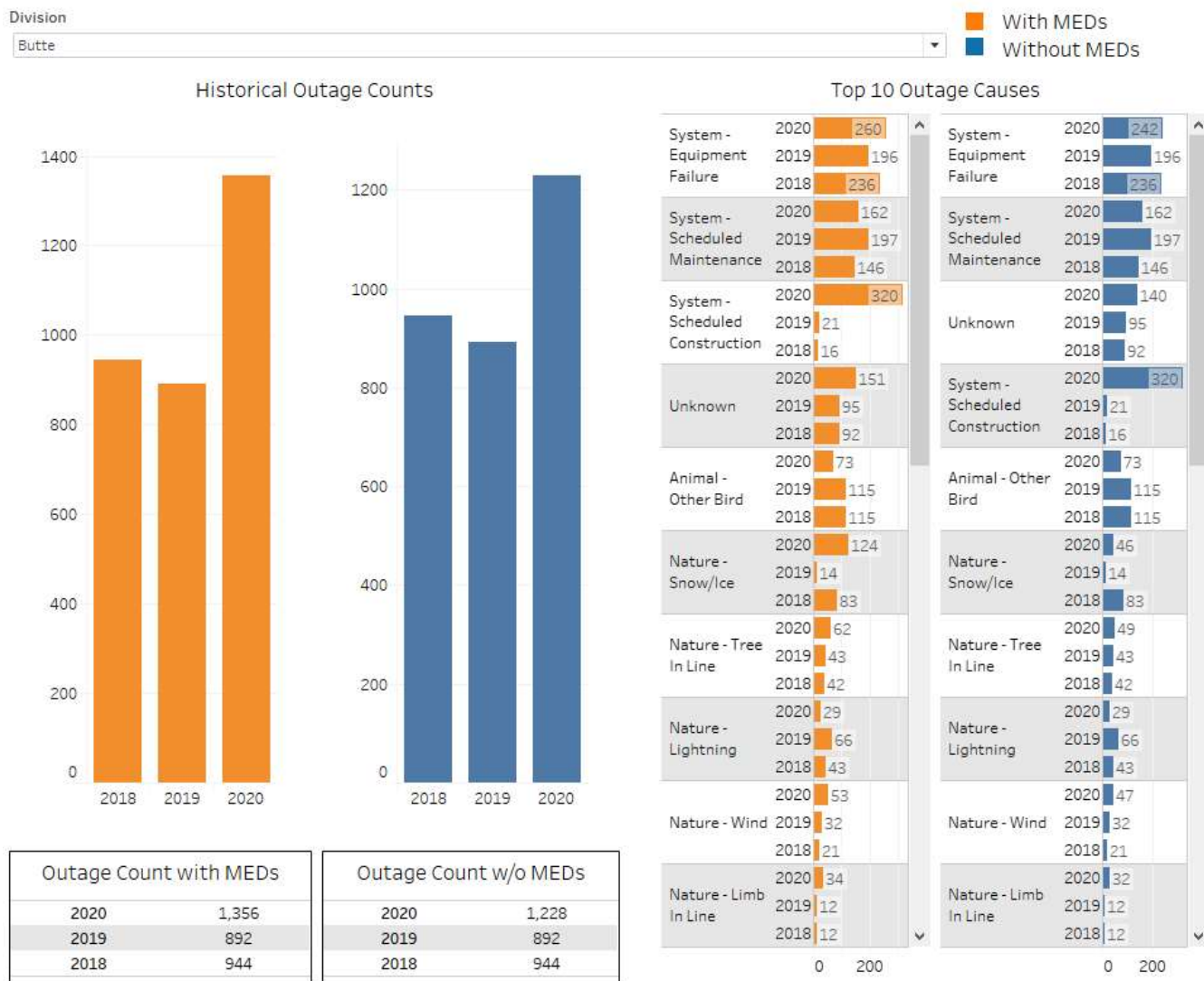
Figure 5.2 Butte system outages by top ten causes with and without major event days (MEDs) as defined in IEEE Standard 1366-2012.
