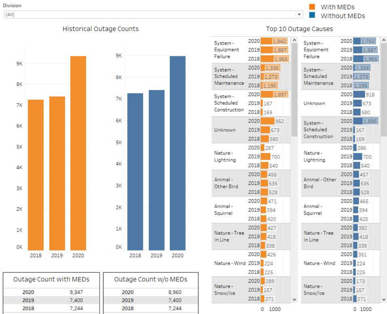
Figure 2.2 Montana system outages by top ten causes with and without major event days (MEDs) as defined in IEEE Standard 1366-2012.
