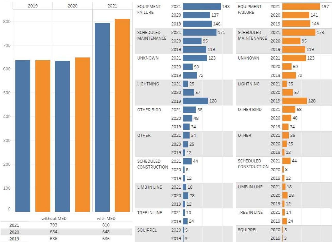
**Figure 7.2** Havre system outages by top ten causes with and without major event days (MEDs) as defined in IEEE Standard 1366-2012.
