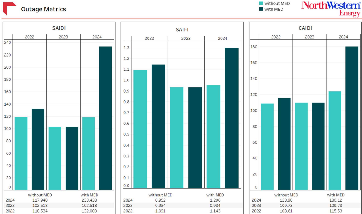
Figure 2.1 Montana system indices with and without Major Event Days (MEDs) as defined in IEEE Standard 1366-2022.
